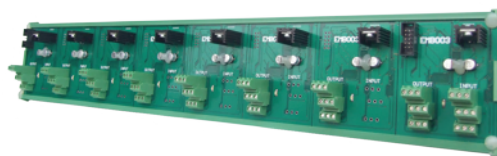
Combination: 1 input and 8 outputs for signal distribution
